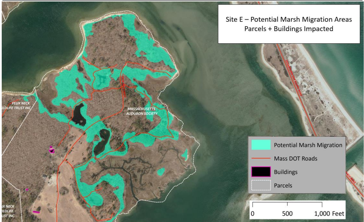
Figure 5. Potential marsh migration areas for Site D (top) and Site E (bottom) showing parcel boundaries and building footprints.
